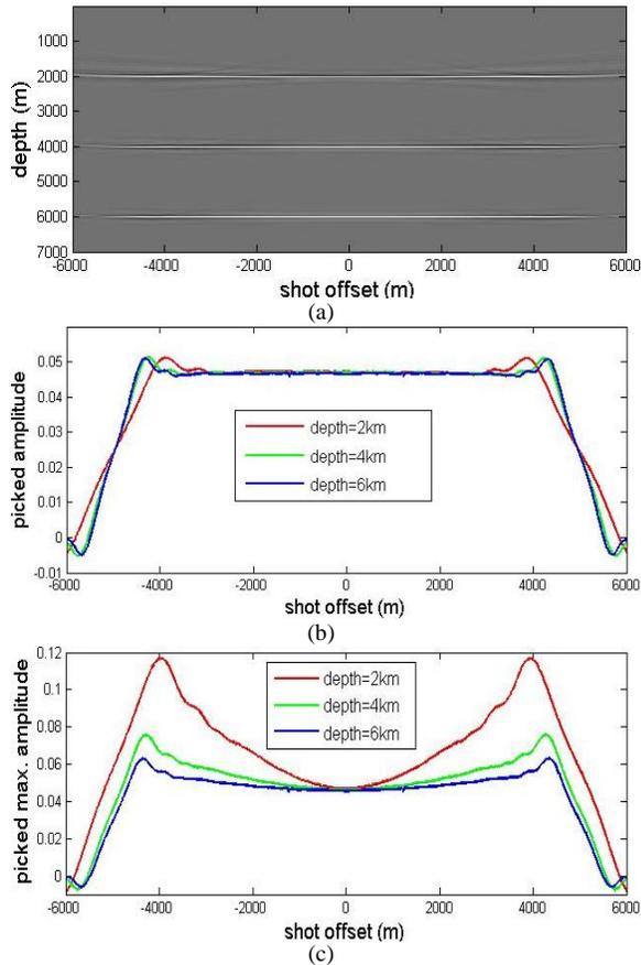
Figure 1: (a) RTM shot image incorporating directional fold correction. The model has 3 horizontal density-contrast reflectors and constant velocity of  $v=3000\text{m/s}$ . (b) Peak amplitude along the 3 reflectors of shot image (a). (c) Peak amplitude of the shot image without incorporating directional fold correction.
