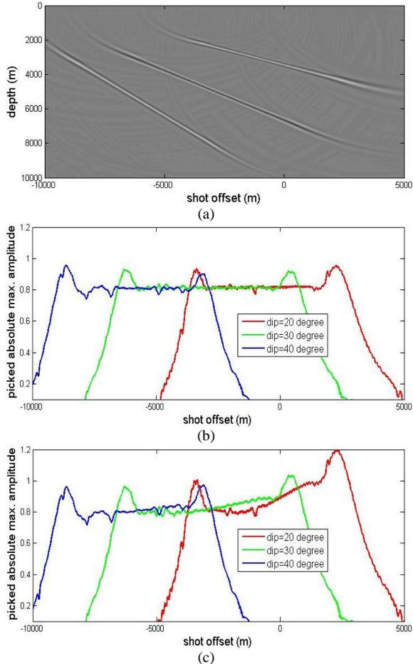
Figure 3: (a) true-amplitude RTM shot image for a  $v(z)$  model ( $v=(2400+0.3z)$ m/s). The model has 3 dipping density-contrast reflectors with the same theoretical absolute reflectivity; (b) Picked peak amplitude along the 3 dipping reflectors of shot image (a); (c) Picked peak amplitude of the shot image without incorporating directional fold correction.
