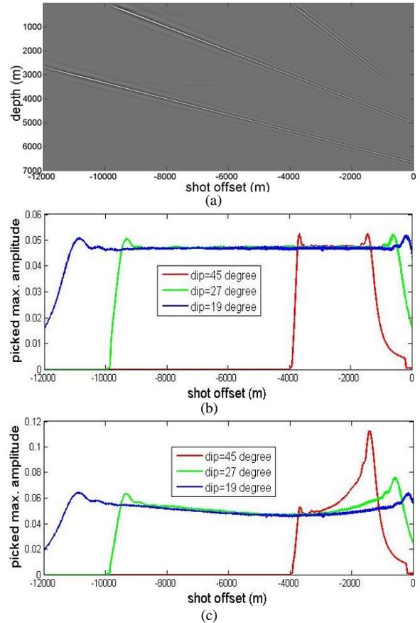
Figure 2: (a) RTM shot image incorporating directional fold correction, for a model with 3 dipping density-contrast reflectors and constant velocity of  $v=3000\text{m/s}$ ; (b) Peak amplitude along the 3 dipping reflectors of shot image (a); (c) Peak amplitude of the shot image without incorporating directional fold correction.
