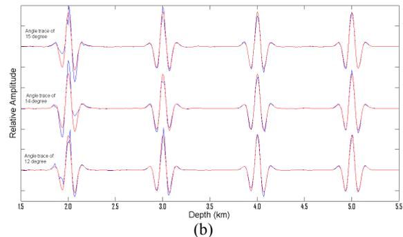
Figure 3. (a) 3D ADCIGs after applying the relative hitcount compensation to the result in Fig. 2a. (b) Comparison of angle traces from before (blue) and after (red) relative hitcount compensation. It can be seen that the under-sampling artifacts in near angles are completely removed for this example.
