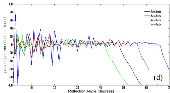
Figure 2. 3D true-amplitude angle gather obtained using shot spacing of 80m $\times$ 80m. (a) RTM angle gather with reflection angle bin of 1 degree. (b) The AVA curves picked along the 4 reflectors in (a). (c) Comparison of actual hitcount number with the theoretical hitcount number for each angle bin at different depths. (d) Percentage error of actual hitcount number with respect to theoretical hitcount number. The same model used in Figure 1 is used here.
