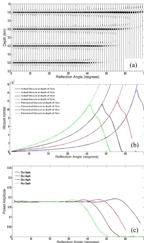
Figure 1. 3D true-amplitude angle gather obtained using shot spacing of 2.5m by 2.5m. (a) RTM angle gather with reflection angle bin of 1 degree. (b) Comparison of actual hitcount number (solid line) with theoretical hitcount
